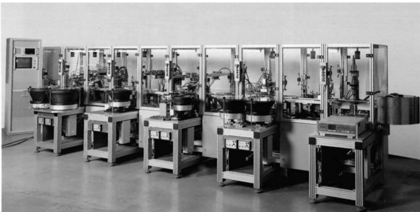
Figure 22 Rectilinear Transfer Machine with High Productivity. (Source: IMA Automation)
