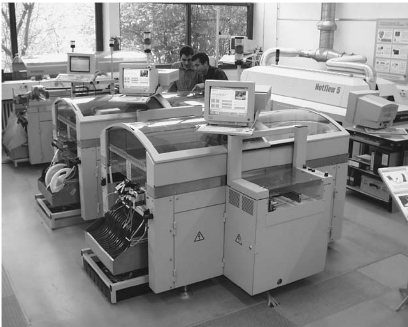
Figure 34 SMT Placement Line (Siemens Siplace).
