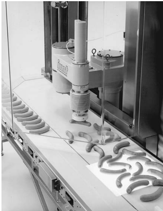
Figure 47 Sorting Sausages with Robots. (Source: imt)
