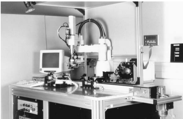
Figure 45 Prototype Assembly Cell for Manufacturing Fiberoptic connectors.
