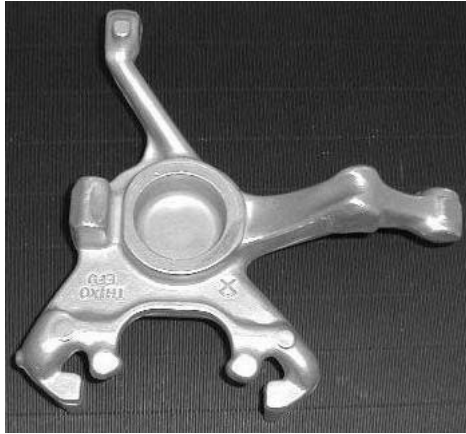
Figure 27 Steering Knuckle Made by Thixoforging. (Courtesy EFU, Simmerath, Germany)
