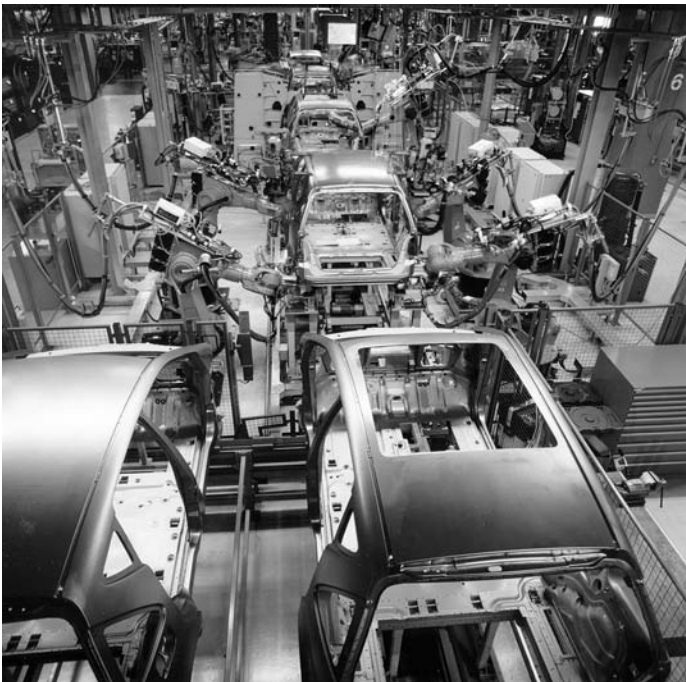
Figure 35 Robotized Spot Welding Line (Source: KUKA Roboter GmbH)
