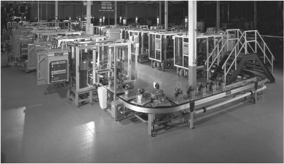
Figure 38 Assembly Line for Large Steering Components. (Source: ATS Inc.)
