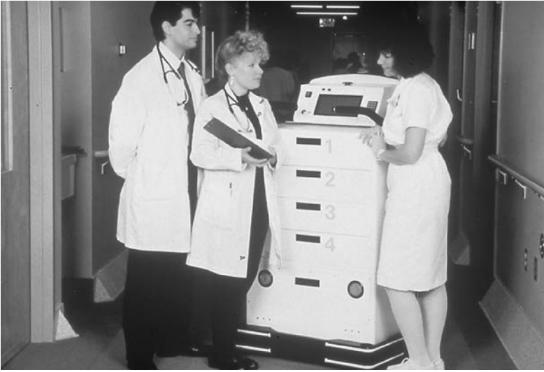
Figure 24 Mobile Robot for Courier Services in Hospitals. (Source: PYXIS)
