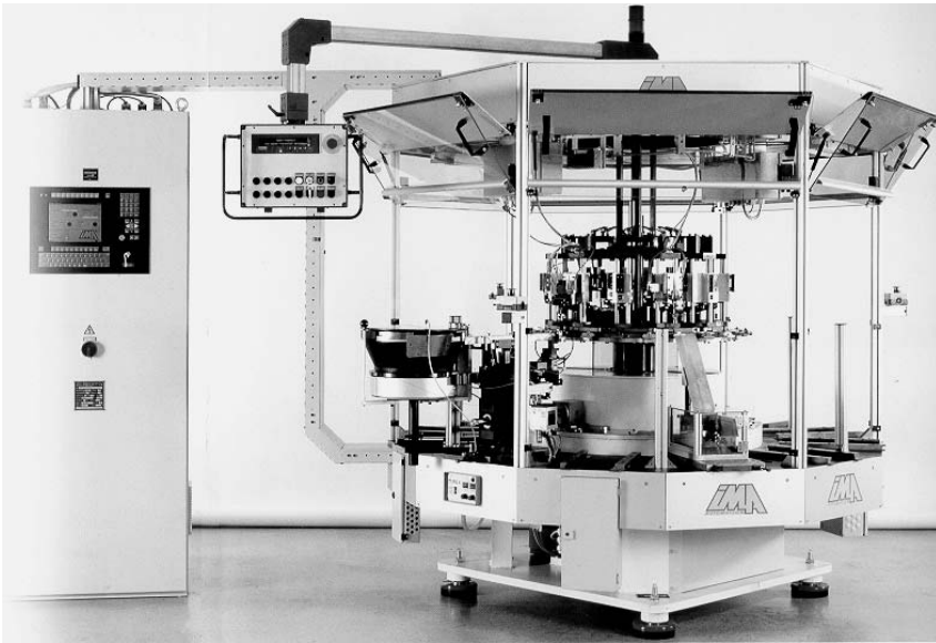
Figure 23 Rotary Indexing Turntable for an Efficient Assembly of Mass-Produced Articles. (Source: IMA Automation)
